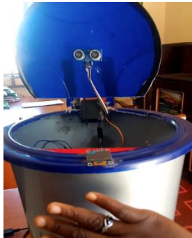
Figure 7: The developed system opened by sensing an object from \pm 2
